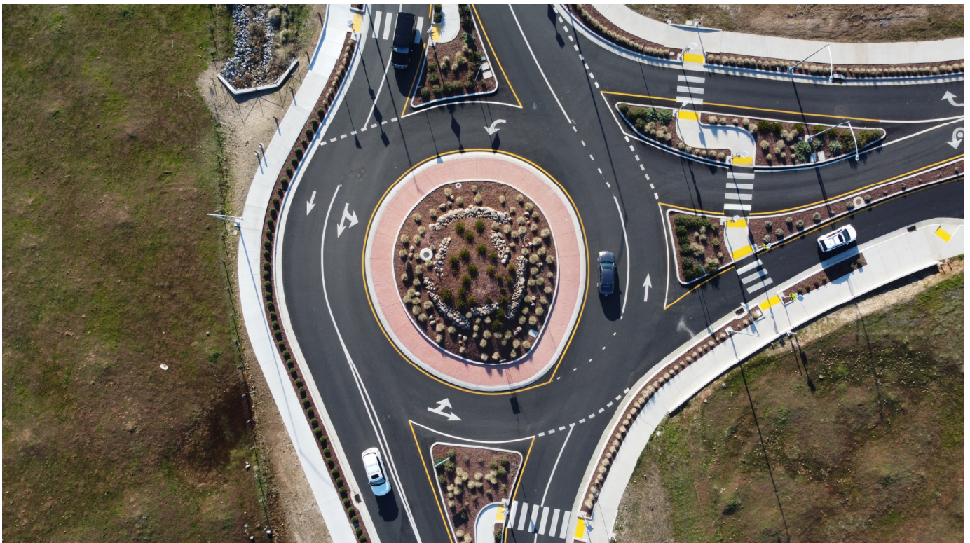
Figure 7-4: Typical Neighborhood Roundabout Entry
