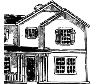
Simple Massing with Gabled Roofs
