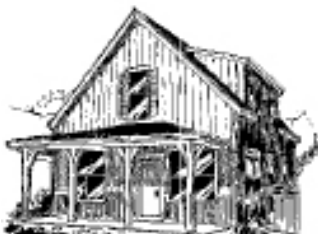
Primary Gable on Front Elevation
