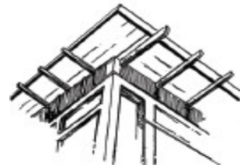
Exposed Rafter Tails
